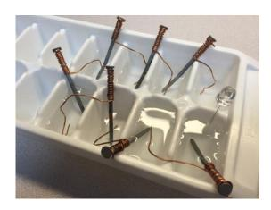
Batteries are made of two different metals – or *electrodes* - suspended in an *acid solution*. With this experiment, our metals are the copper (wire) and the zinc (galvanization of the nail). The acid is contained in the vinegar.
