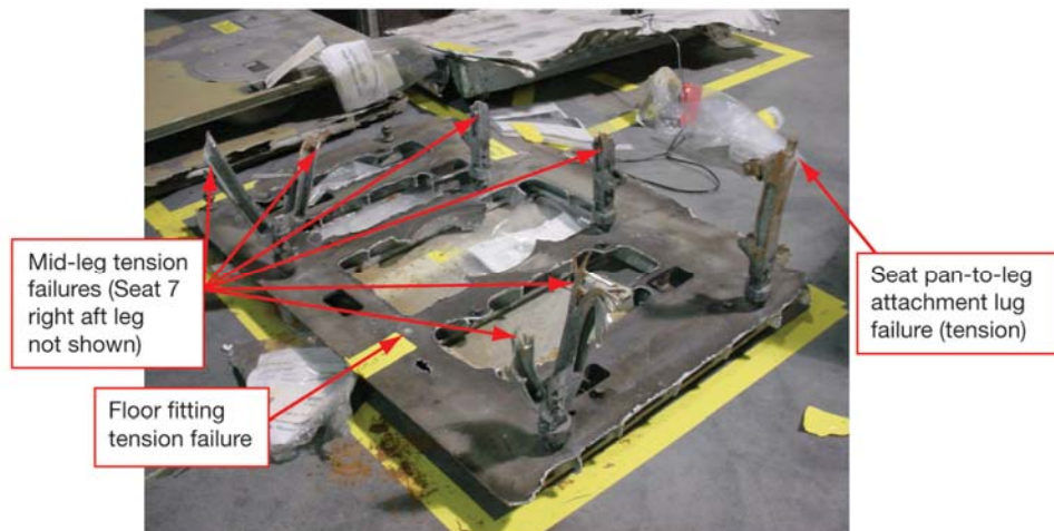
Figure 3.1-14. Recovered lithium hydroxide door with seats 6 and 7 legs attached.
