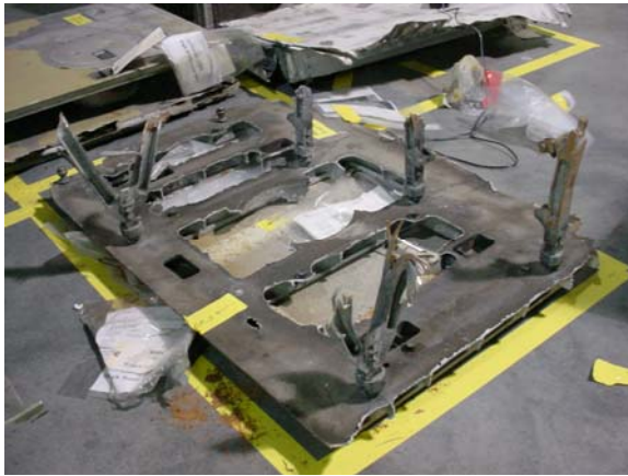
Figure 2.1-33. Recovered lithium hydroxide door with some seat legs still attached.
