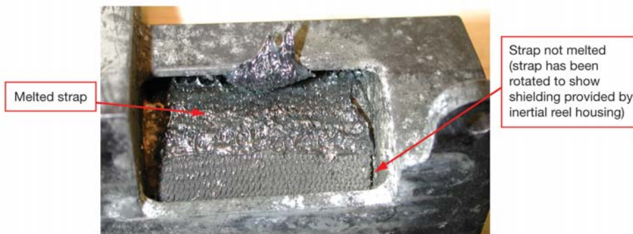
Figure 3.1-24. Close-up of strap melt pattern.
