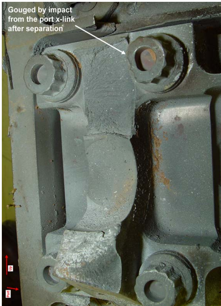
Figure 2.2-47. Columbia Reconstruction Database debris item no. 2207, which includes the remainder of the lug fitting that supports the aft end of the port x-link.
