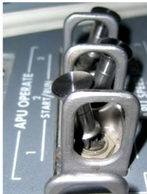
Figure 3.4-12. Operation of the lever-lock controller switches (side view).
