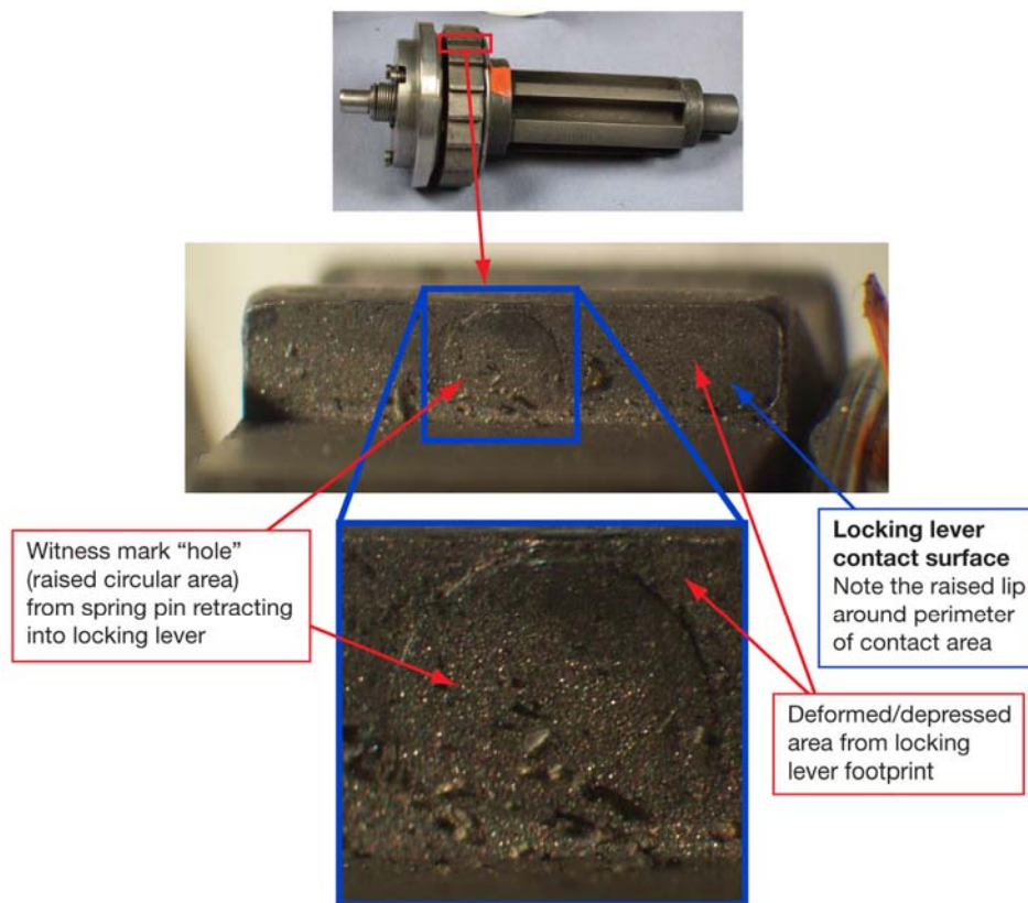
Figure 3.1-33. Inertial reel locking gear witness mark.
