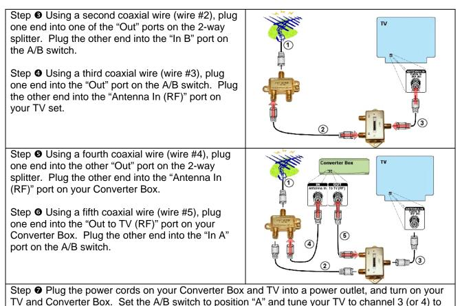
Step ♥ Plug the power cords on your Converter Box and TV into a power outlet, and turn on your TV and Converter Box. Set the A/B switch to position "A" and tune your TV to channel 3 (or 4) to watch digital TV. Using the remote control that came with your Converter Box, follow the on-screen set-up guide to scan for available DTV channels, and begin enjoying the benefits of Digital Television! To watch analog TV, set the A/B switch to position "B" and change the channel on your TV set.
