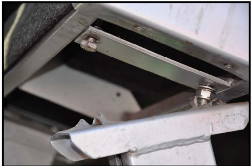
Seat separation from the outboard pedestal. CF-023-10 07-29-10 DH-A (7) cropped
