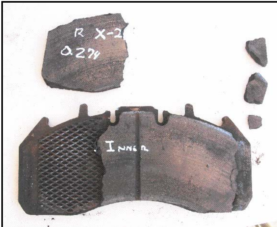
Right inboard brake pad of axle 2 of Vehicle 2 (MCI). CF-023-10 07-27-10 SP (54) cropped
