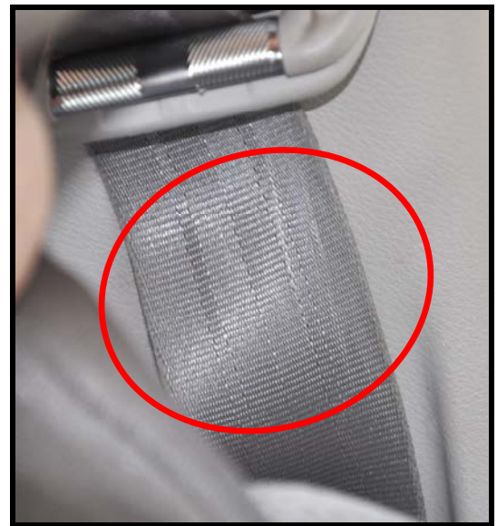
Waviness to restraint webbing. CF-023-10 07-27-10 DH-A (100) (cropped)
