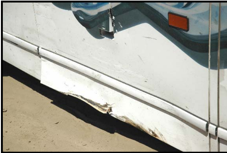
Fractured lower edge of baggage access door 3. CF-023-10 07-26-10 DN-B (10)
