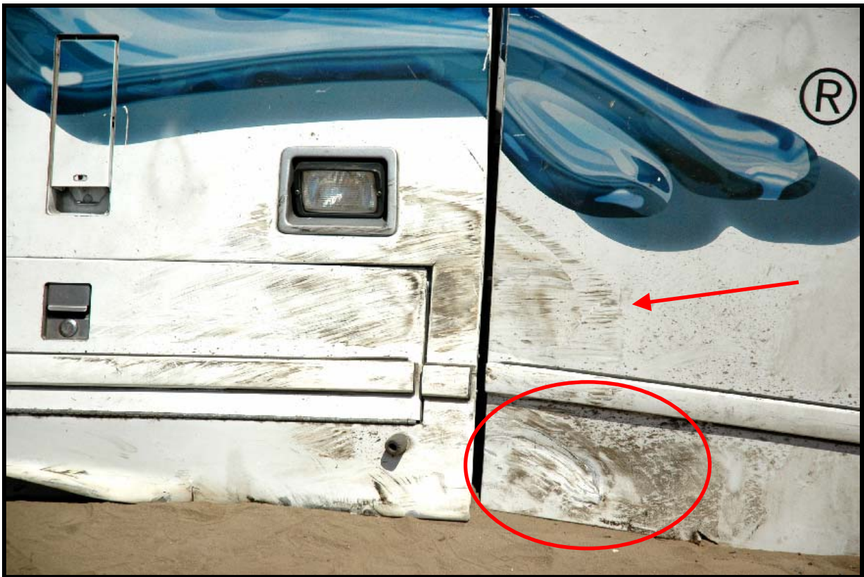
Black transfers and contact damage to baggage access doors 1 and 2 of Vehicle 2 (MCI). CF-023-10 07-26-10 DN-B (5)
