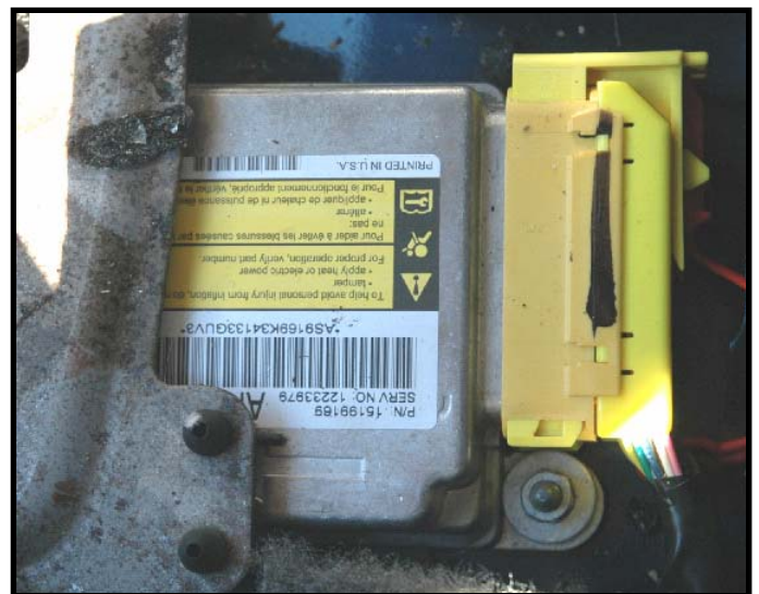
The SDM mounted in Vehicle 1 (Chevrolet). CF-023-10 08-03-10 JK (7) cropped
