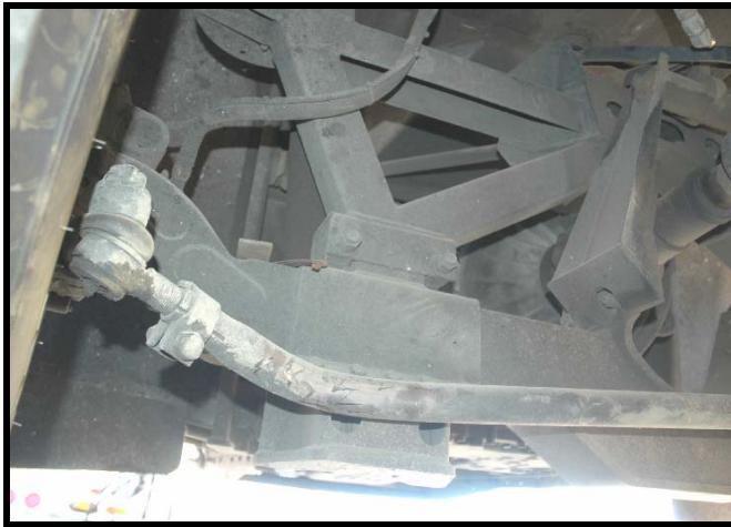
Bent right side drag link of Vehicle 2 (MCI). CF-023-10 08-06-10 MS (41)
