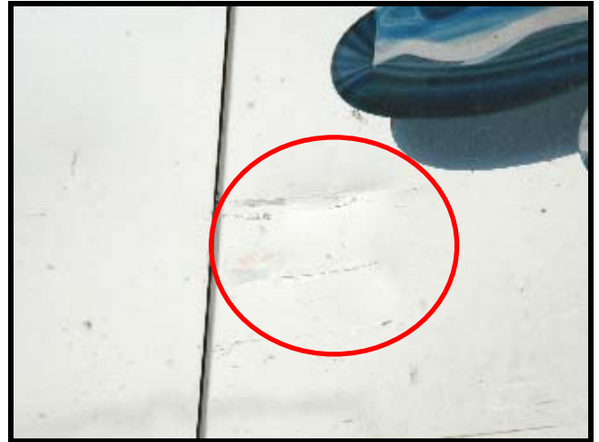
Blue and red transfers on baggage access door 3. CF-023-10 07-26-10 DN-B (12) cropped
