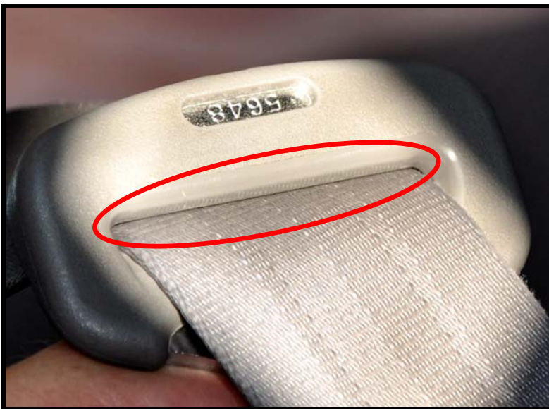
Latch plate imprinting. CF-023-10 07-27-10 DH-B (6) (cropped)
