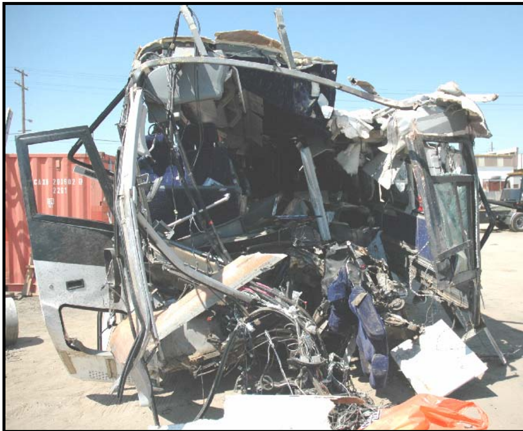
Damage to the front of Vehicle 2 (MCI). CF-023-10 07-26-10 DN-B (51) (cropped)
