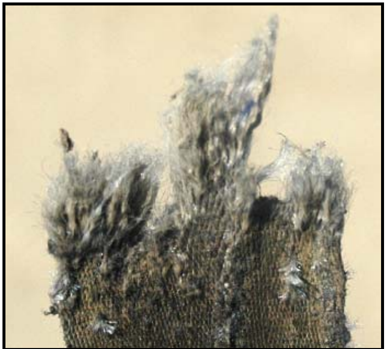
Torn restraint webbing. CF-023-10 07-27-10 DN (39) (cropped)
