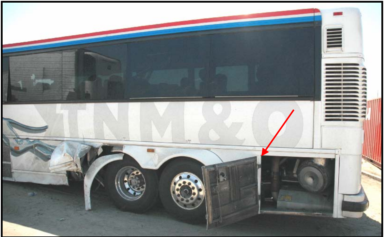
Left side damage to Vehicle 2 (MCI). CF-023-10 07-26-10 DN-B (30) cropped
