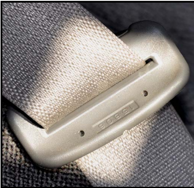
Angular abrasions on latch plate loop guide. CF-023-10 08-02-10 DH (58) cropped
